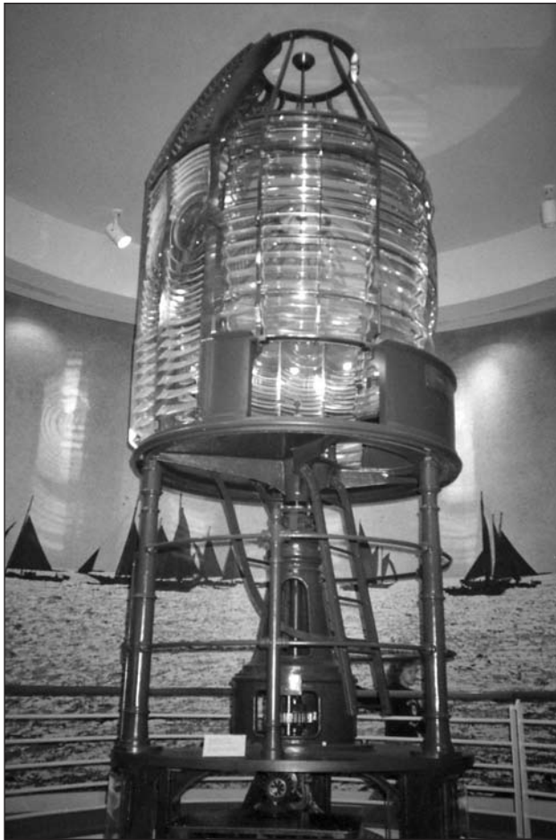
The Cape Charles First Order Fresnel lens at the Mariners' Museum in Newport News, VA. Photo by Rete Williams.
